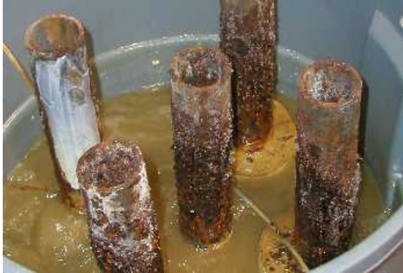
FIGURE 4 – Aerated Salt Bath
