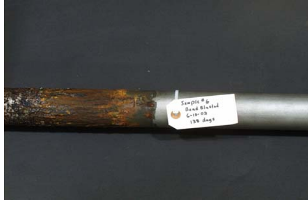
FIGURE 5 – Pipe after 138 Days of Exposure
